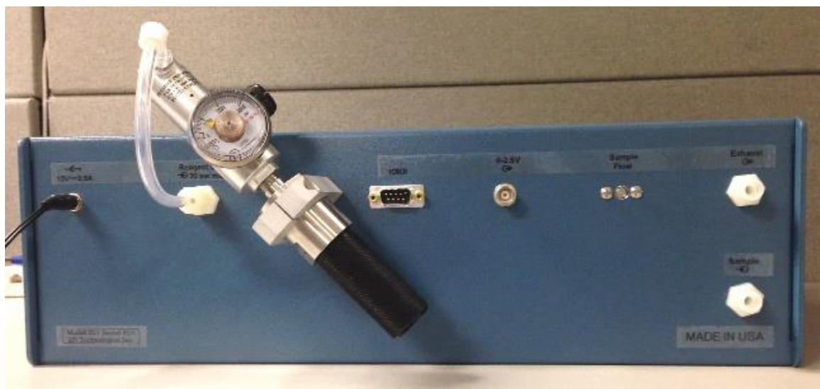
FIGURE 10.4. Top: Back of Model 211 Ozone Monitor. Bottom: With the N 2 O Cartridge Cracker in place.
