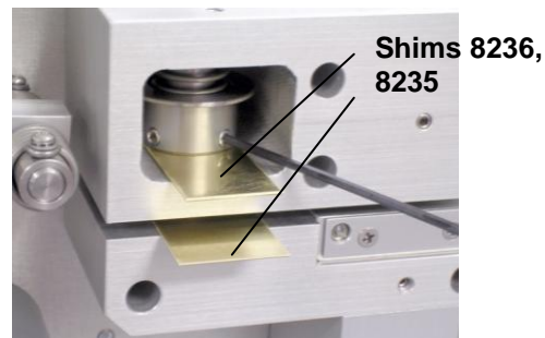
Using Shims for Reassembly
