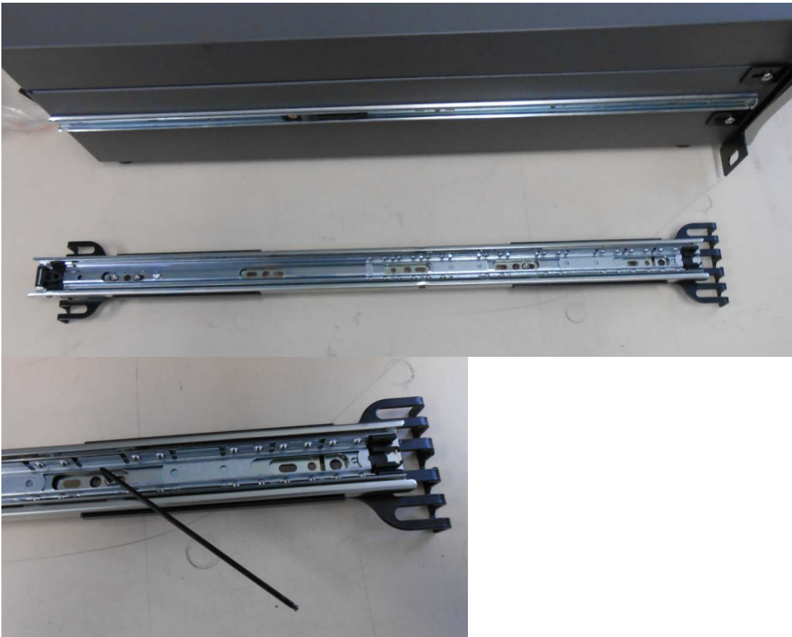
Figure 69 – Attach Rack Mount Adaptors to Outer Slides
