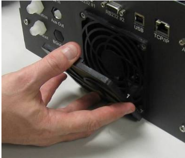
Figure 54 – Removing the Fan Filter
