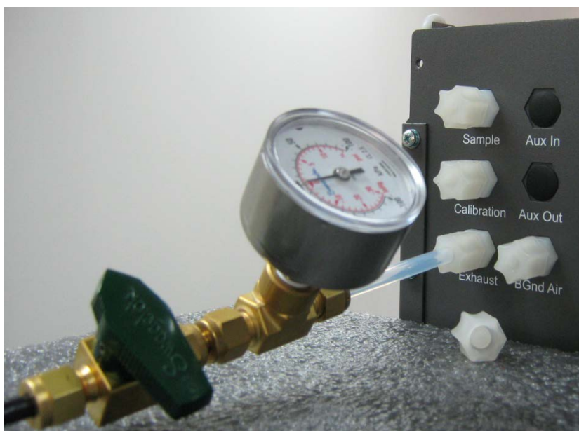
Figure 56 – Leak Test Jig on Exhaust
