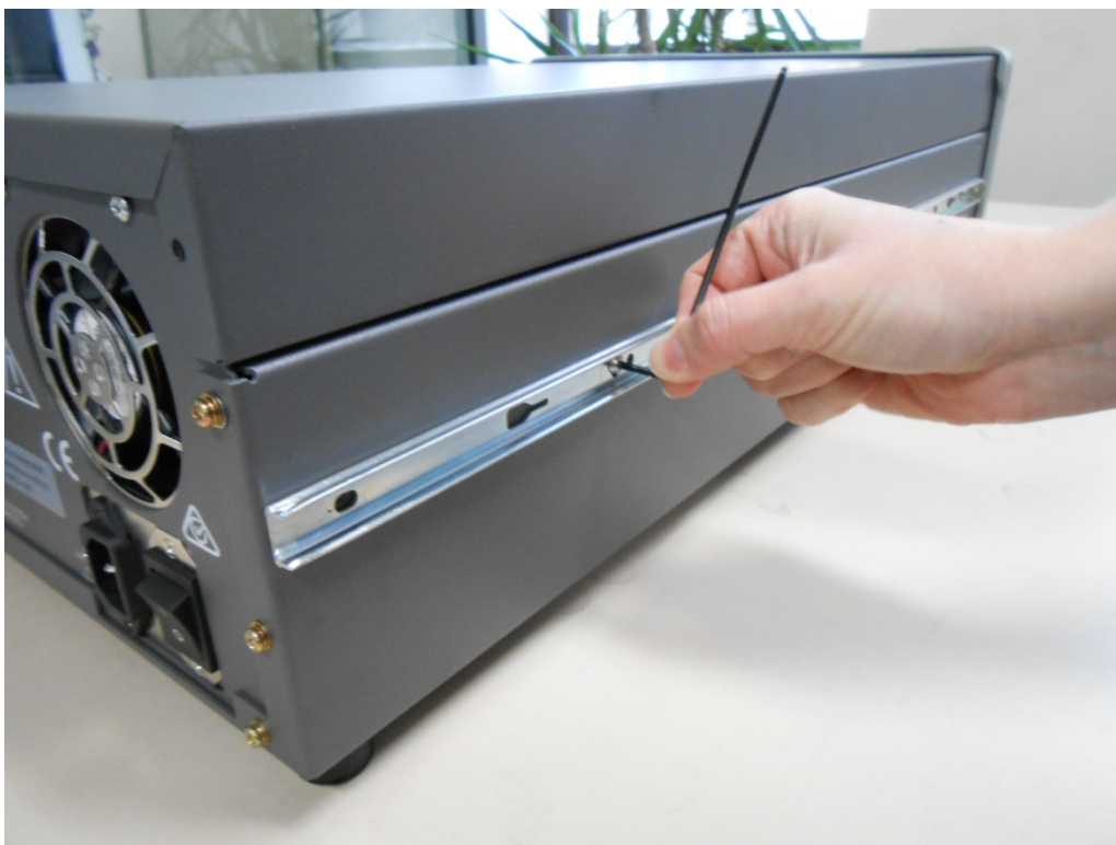
Figure 67 – Assemble Inner Slide on Chassis
