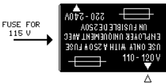
Figure 2.2. Fuse holder, here set at 115 V mains supply.
