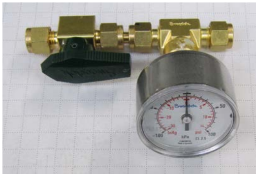
Figure 52 – Leak Test Jig – (PN: H050069)
