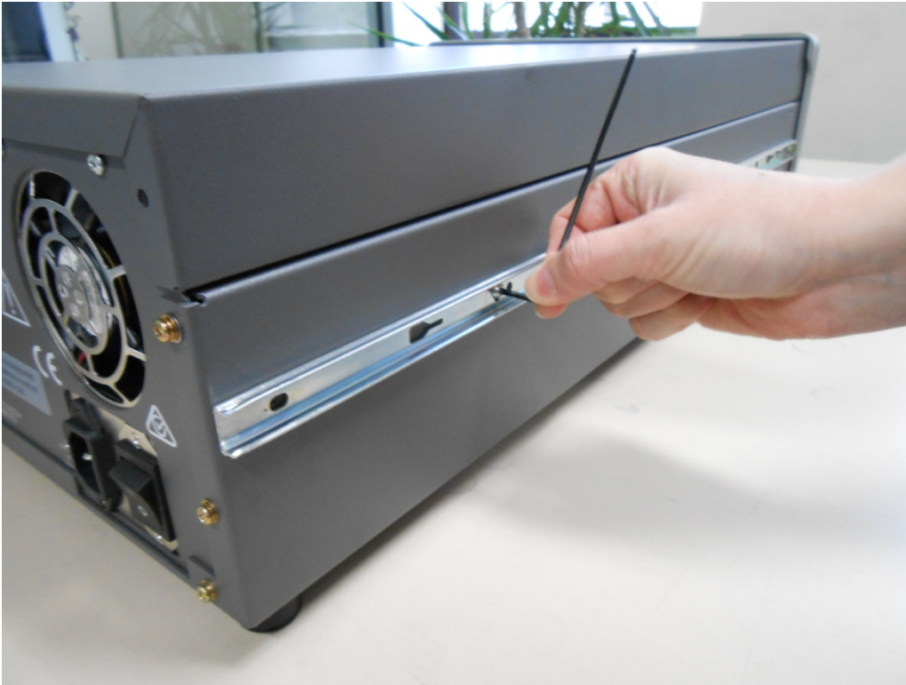
Figure 71 – Assemble Inner Slide on Chassis
