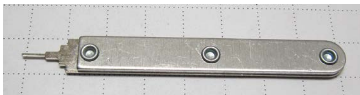
Figure 50 – Minifit Extraction Tool – (PN: T030001)
