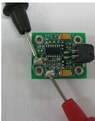
Figure 61 – Test Point Location
