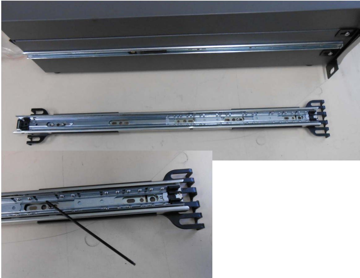
Figure 73 – Attach Rack Mount Adaptors to Outer Slides
