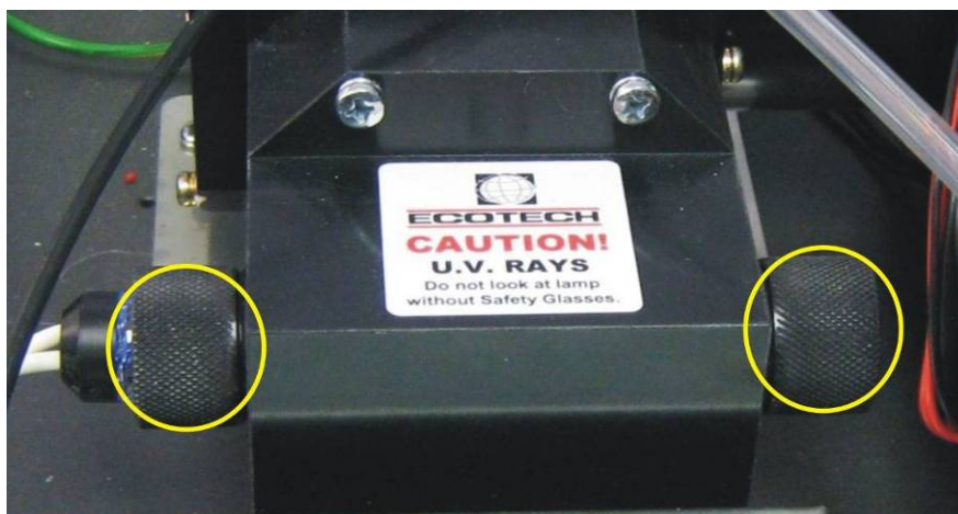
Figure 60 – Collets of the UV Lamp
