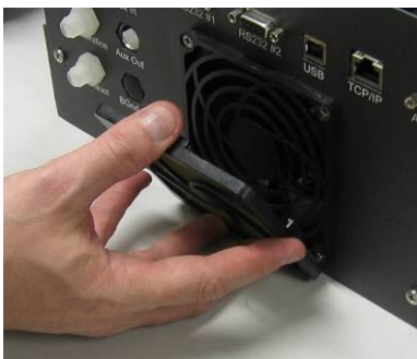
Figure 55 – Removing the Fan Filter
