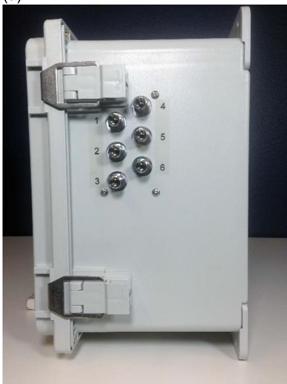
Figure D-7. (a) Side View of the Model 106-L-MC6 Multi-Channel Ozone Monitor. (b) Top inside view, with filter installed (see Figure D-5 for component labeling).
