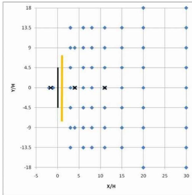
Schematic representation of the experimental plan showing the locations of the line source release on the left (bold), the barrier (orange), bag samplers (blue diamonds), and sonic anemometers (x). H is the height of the barrier which was 6 m.
