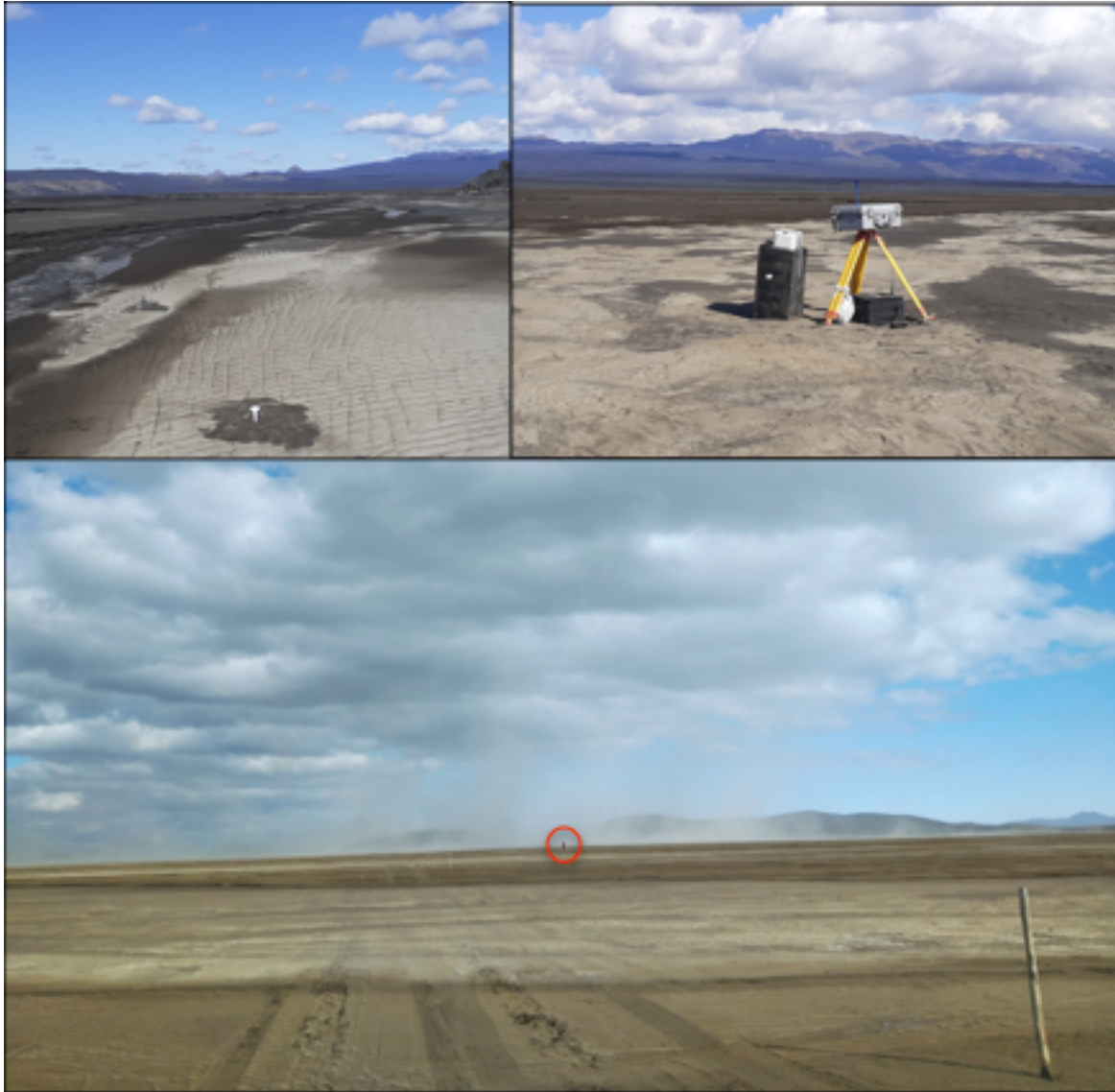
Figure 3. Sediment, suspended dust and aerosol samplings at DYN (64° 54' 28.3428" N 16° 39' 4.1544" W). The red circle marks the Grantee while sampling. Peak dust concentrations of 400 \mu\text{g m}^{-3} were captured by the DustTrak monitor, but the concentrations were likely significantly higher in the center of the dust storm.
