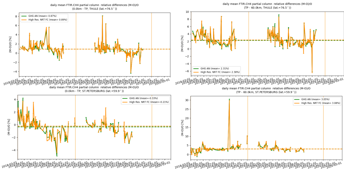
Figure 10.3.2: Daily mean of relative differences for tropospheric CH 4 columns (left) and stratospheric CH 4 columns (right) at Thule (top) and St. Petersburg (bottom). At Thule the stratospheric column shows a reduced bias during the summer months, while at St. Petersburg the tropospheric column performs worse during June-October.
