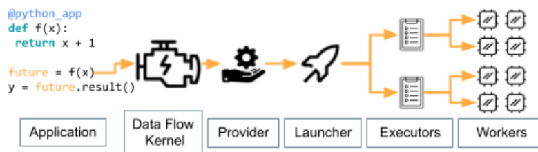
Figure 3.2: High level schema of the Parsl architecture. Image from the “Parsl 1.3.0-dev documentation – Quickstart” (2026).
