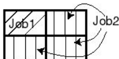
(b) Job2, submitted but can't start since it needs 4 processors. Remaining 3 reserved by Job2.
