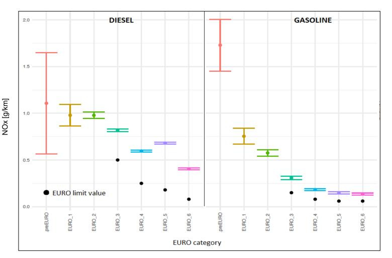
**Figure 3**: Comparison of observed and EURO emission limits for cars (AMB 2017).
