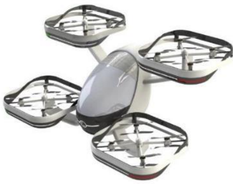
Figure 1-4: Render of TECNALIA's Air Taxi design (left) and the operational prototype presented in San Sebastian (Spain) in July 2019 (right).
