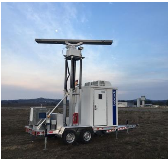
Figure 1-8: LUA Ground Mobile Unit primary and secondary radar (left) and air traffic coordination diagram of LUA system (right)
