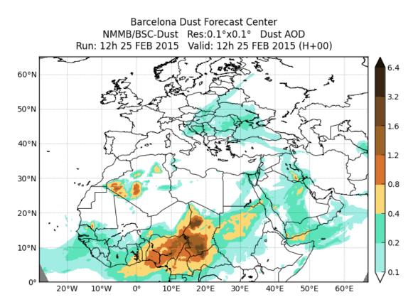
Figure 1. Domain of simulation of the NMMB/BSC-Dust model. The colour scale shows AOD (at 550nm) forecast on 25<sup>th</sup> February at 12h.
