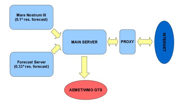
Figure 2 System architecture of the BDFC.
