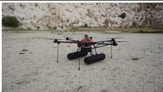
Figure 2: Custom drone with small embedded lightweight air pollution sensors
