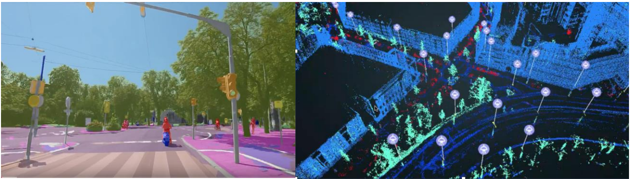
Left: Semantic segmentation automatically generated by Mapillary's algorithm. Right: Semantic point clouds generated using only monocular images
